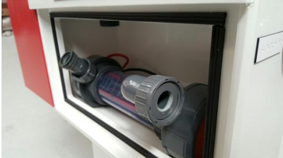
7.1.6 Attach the PVC pump discharge hose to one end of the cell. Connect the drain hose to the other connection and place the open ended hose into the bucket of prepared acid solution.
